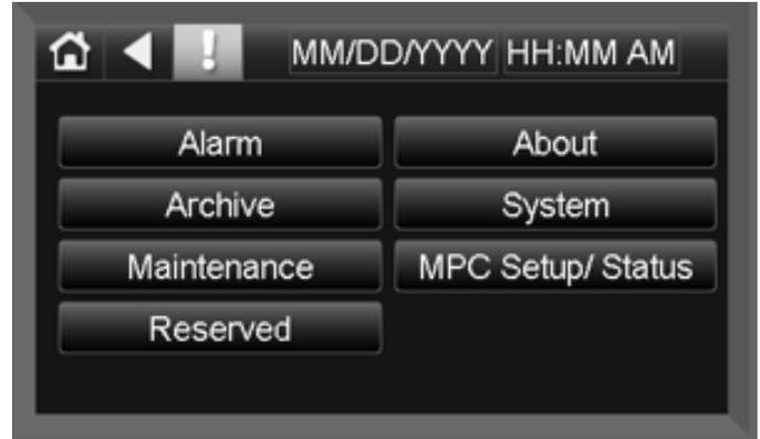
There are three Icons that are present on every screen, Home, Back and Information. Clicking the Home Screen Icon will return the user to the screen which is the top of the Screen Hierarchy. The back arrow Icon is used to go up one screen in the hierarchy. The Information Icon displays any active alarms or other pertinent system information
