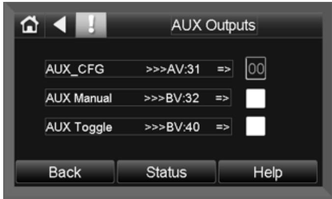
1. **AUX\_CFG** - Controls the output function of the AUX output dependent on the value of AV: 31. See table to the right.
