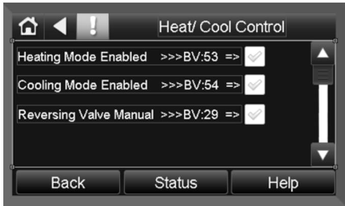
1. **Heating Mode Enabled**- When “Heating Mode” is checked, Heating Mode is enabled. The default is checked. This allows Heating Mode to be disabled when cooling only is desired.
