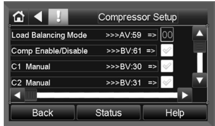
1. **Load Balancing Mode** - Defines the mode of operation for the runtime balancing of a 2 Compressor application. The modes are set by entering the following in AV:59
