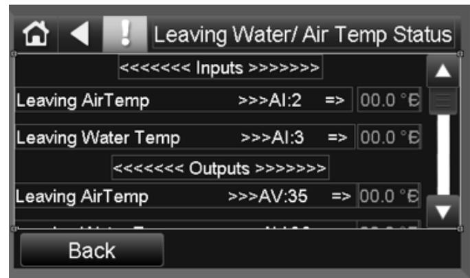
1. **Leaving Air Temp**- Reports the Leaving Air Temp when an appropriate sensor is connected to AI:2.
