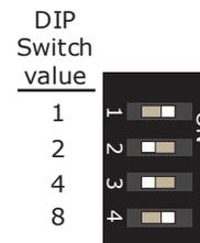
**EXAMPLE:** DIP switches 1 and 4 above are on. Their values (1 + 8) total 9, so the sensor's address is 9.
