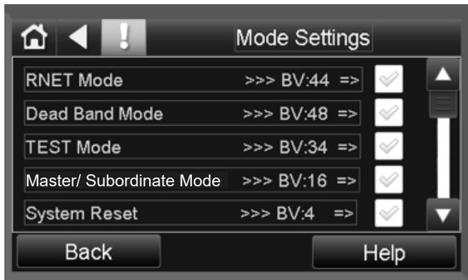
1. **RNet Mode**- allows the MPC to function with LStat Sensors when RNet is OFF. Also allows monitoring of inputs 5 and 6 (temp or dry contact) when a RNet sensor is used.
