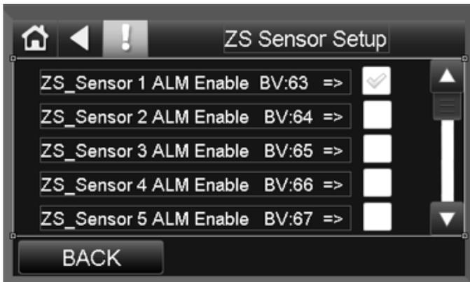
1. **RNet Sensor 1 Alarm Enable**- Checking this will tell the sensor alarm logic to expect a valid sensor to be present at Address 1. If it is not present, a Sensor Not Present Alarm will be generated. This is required because the unit can have up to 5 zone sensors and is set to look for all 5 even when only one or two are present. (It is normally defaulted to checked.)
