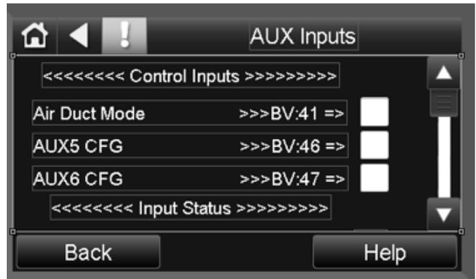
1. **AUX5 CFG** - Determines if AUX5 is set for Temperature or Dry Contact Input.
