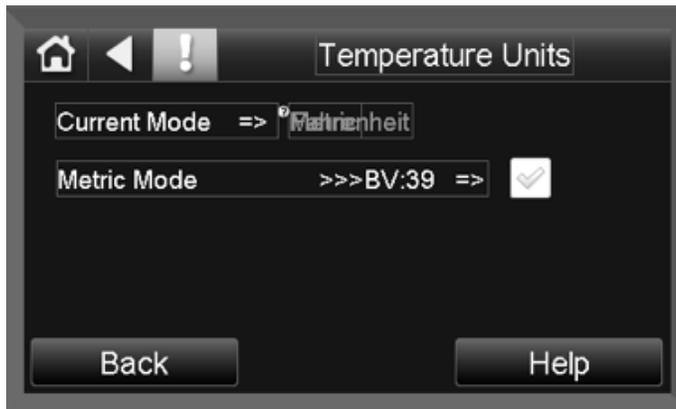
1. **Current Mode** - displays the current Temperature Mode as Celsius or Fahrenheit.
