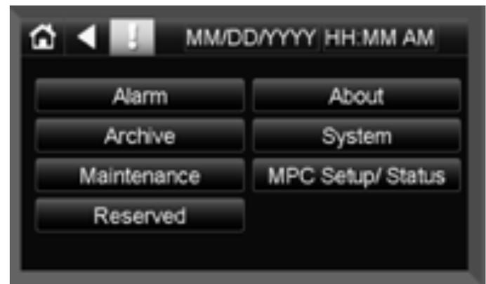
4. Navigate to the "Sensor Setup and Status" screen by pressing **<MPC Setup/Status>** then **<Sensor Setup/Status>** buttons. Press the **<ZS Sens Active>** button. This should display the correct address and number of ZS Sensors that are attached to the MPC. Press the **<Back>** and go to the "ZS Sensor Setup" screen where you will enable the alarms for each sensor installed and detected in the previous step.
