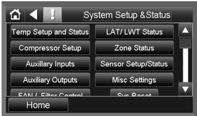
1. **Temp Setup and Status**- Provides user access to Temp Units and Temp Setpoints screen for setting temperature units and temperature setpoints respectively. There are no control or status points on this screen.
