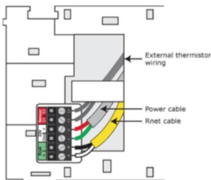
7. Attach the backplate to the wall or panel.
