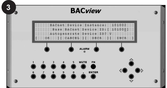
The device instance is typically six digits long. The last two digits correspond to the addressing rotary dials so these should not be changed using the BACview6.
