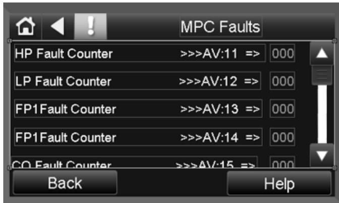
1. **HP Fault Counter**- High Pressure fault counter.
