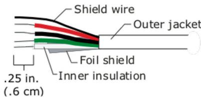
6. Strip about .25 inch (.6 cm) of the inner insulation from each wire.
