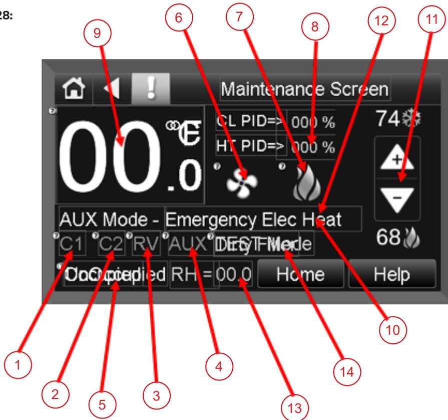
1. Compressor Stage 1 "ON" when → C1 icon is visible.
