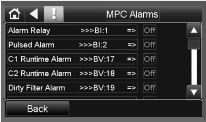
1. **Alarm Relay**- Monitors the Alarm Relay Input BI:1 from DXM2, EXM etc.
