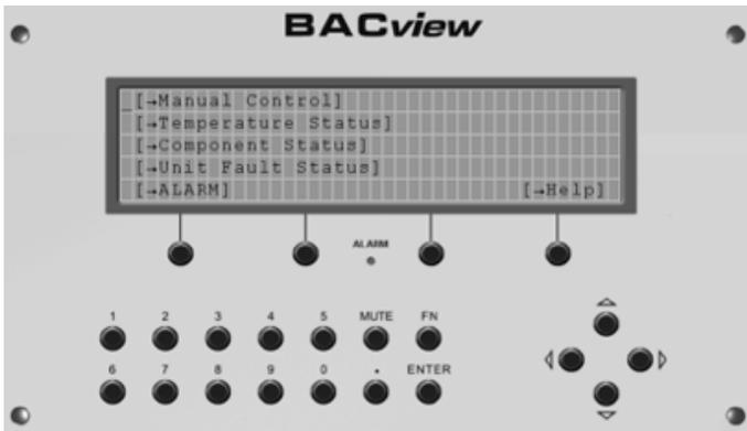
4. Navigate to the "Sensor Setup and Status" screen by highlighting **[Manual Control]** and clicking **<Enter>**, then highlighting **[Unit Control]**, and clicking **<Enter>**. Scroll down the list and make sure the following are set correctly.
