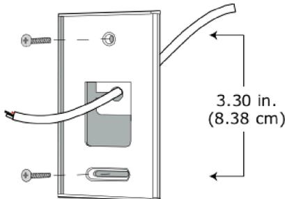
4. Use 2 screws to mount the backplate to the wall or outlet box.
