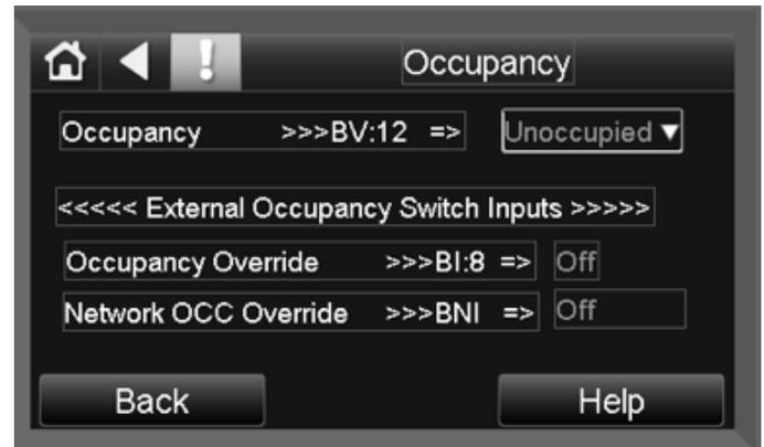
1. **Occupancy** - This point controls whether the unit is in Occupied or Unoccupied Mode. It is normally defaulted to Occupied. It can be set and overridden via the Equipment Touch or from the BMS control program (WEBCTRbn L).
