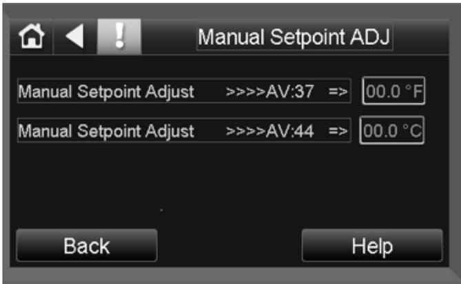
1. **Manual Setpoint Adjust (AV:37)** - Sets the Adjustment span when in Fahrenheit Mode.
