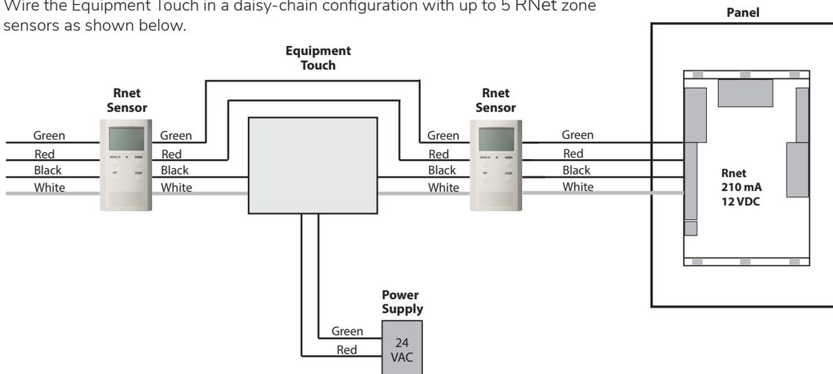
**Note-** The Equipment Touch does not require the user to set an address for it.
